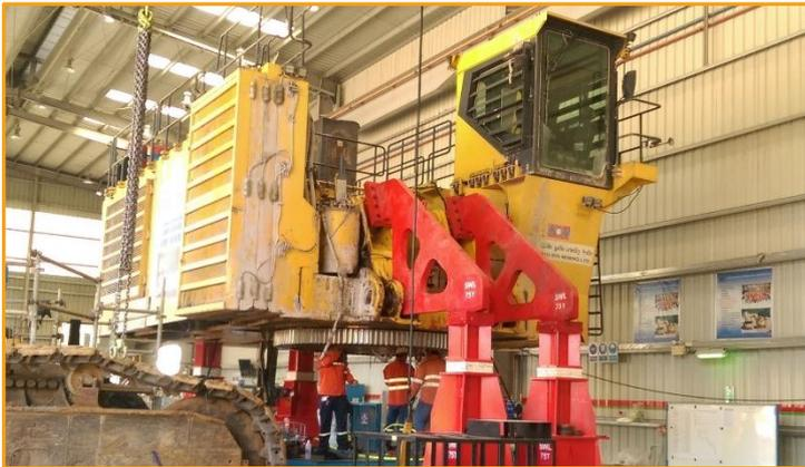
*A PC3000 lifted from the carbody by the custom-built 'banana link' jacking stand. The jacking system is used to replace slew rings in the PC3000 face shovel and PC 2000 excavator fleet inside the Phu Kham Copper-Gold Operation's mobile maintenance workshop.*
